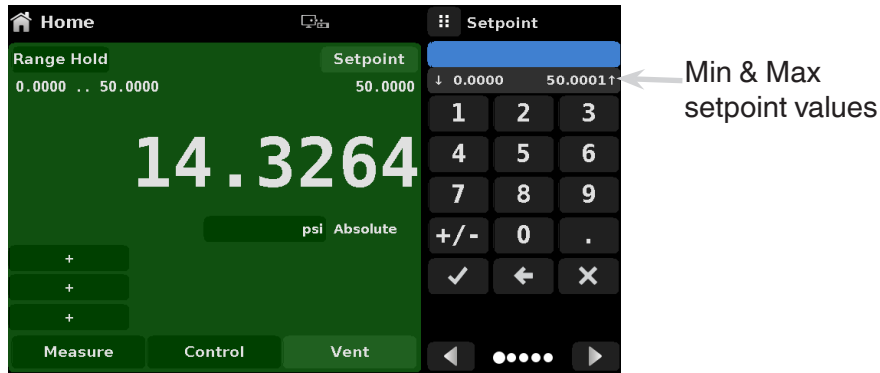
Figure 6.4.1.2.1 – Numeric Keypad Setpoint Entry
