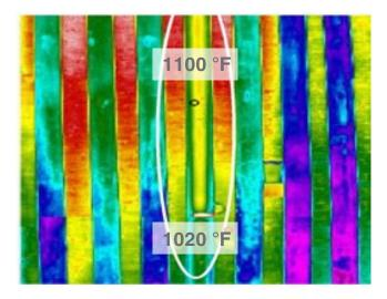
In the above image, the upper two-thirds of the middle furnace tube (circled) shows extensive coking. We know this because the IR scan reveals the coke signatures, and the temperature is around 1100°F. Meanwhile, the TSTC, installed lower on the tube, registers 80°F lower.
