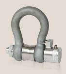
The F5302 is a load-measuring shackle for static and dynamic tensile force measurement. The force transducer is a high-strength stainless steel load pin with welded-on thin-film sensor elements. The dimensions and handling of the F5302 shackle correspond to those of standard shackles. Thus a universal application, even in existing systems, is guaranteed.
