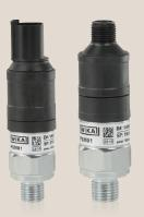
The PSM01 is the economical solution for implementing switching functions in mobile working machines. It is a high-quality, snap-action switch with self-cleaning contacts and can be delivered as a normally closed, normally open or change-over switch. Its switch point can be individually and easily set via an adjustment screw. The compact design of the PSM01 also enables mounting in hard-to-access locations, particularly with a socket wrench.
