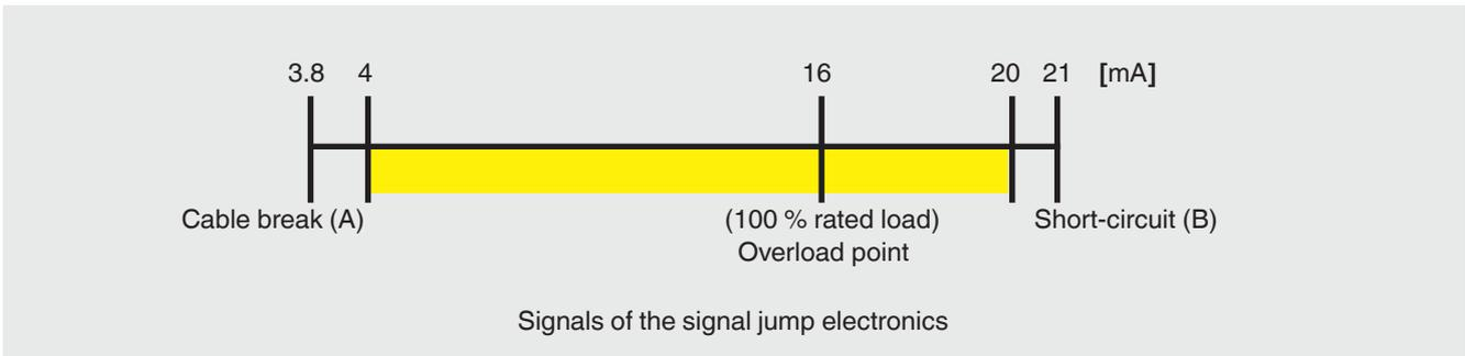
With a fixed signal jump of, for example, 4 mA, the test cycle can then be triggered, in any operating state, by activating the test relay. The upper measuring range limit of 20 mA will never be reached and thus the checking of the signal jump is enabled.
