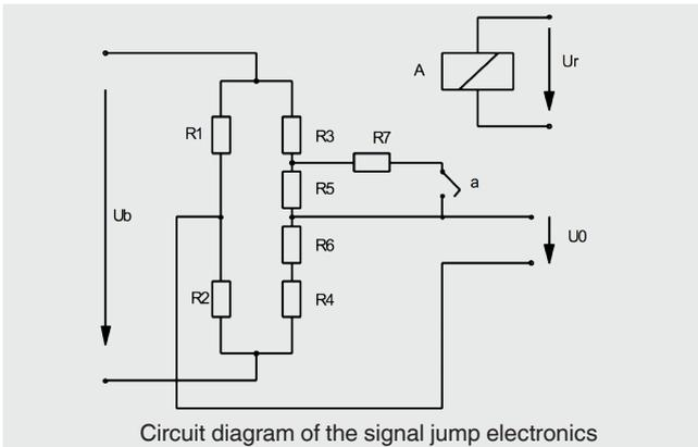
With these force transducers, four variable resistors (R1 ... R4) are connected together to form a Wheatstone bridge. When the measuring body deforms, the opposing resistors are stretched or compressed in the same way. This leads to a detuning of the bridge and a diagonal voltage  $U_0$ .
