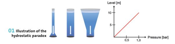
A static liquid generates, through its specific density and the acting force of gravity, a corresponding weight force or hydrostatic pressure which increases proportionally with the filling height. Consequently, the hydrostatic pressure represents a direct measure of the fill level or degree of filling of a tank or vessel.
