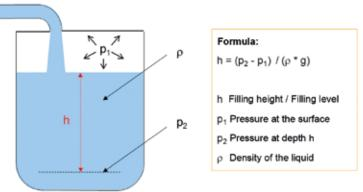
03 Level measurement in sealed, gas-tight tanks and vessels
